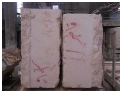
Figure 1: Stone blocks prepared for cutting into slabs using gang saw machine
